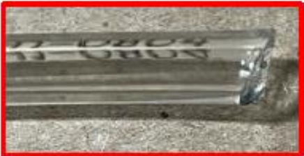
Angled cut on tube end
