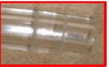
Gouged surfaces on the flexible tube (area inserted into the PTC)
