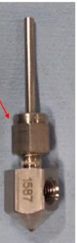
Tighten seal nut: finger tight + 1/4 turn MAX
