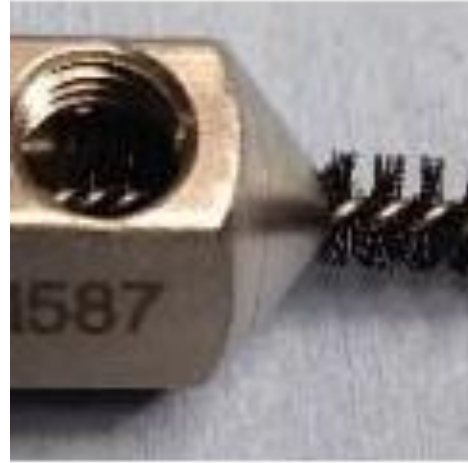
Brush inside the nozzle bore (both ends), female thread, and inside the central cavity
