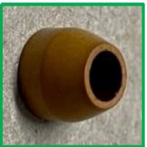
Functional Ferrule: smooth surfaces, clean edges
