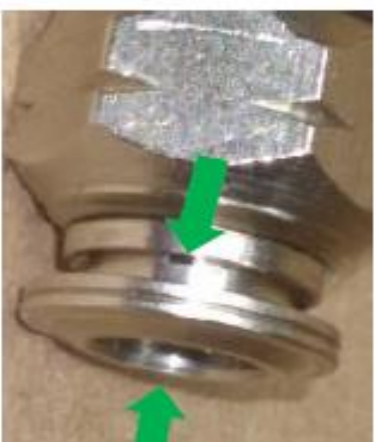
Release collar must move freely (Fully press in and return on its own)
