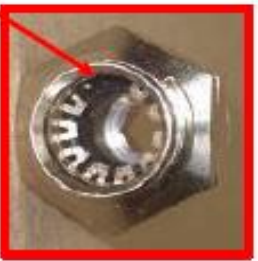
Damaged retention teeth
