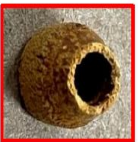
Leaking Ferrule: pitted and chipped surfaces (cleaned with harsh chemicals)
