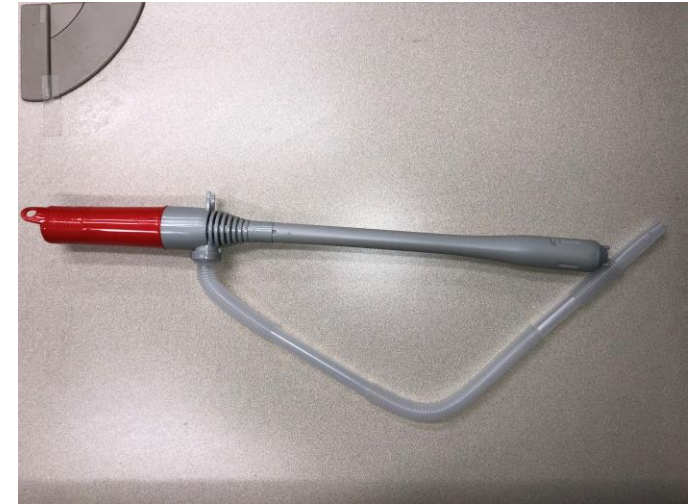
Sealant Transfer Pump
