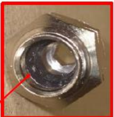
PTC Contamination on the O-ring
